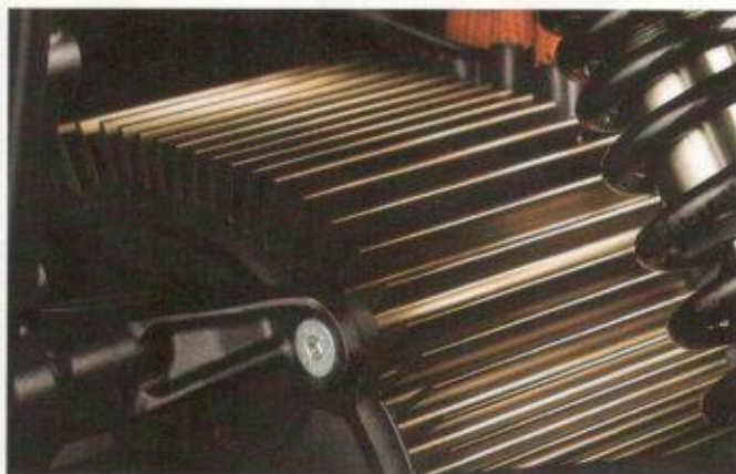
Most of where the engine compartment would normally be is now battery, and the engine is this unit found near where the swingarm meets the frame. It's called a Z-Force 75-7 passively air-cooled, high efficiency, radial flux permanent magnet, brushless motor, which we hope is good. It pushes 54 hp, but more importantly it pushes 92 Nm torque, which is available instantly thanks to no clutches and gearbox and other things that get in the way.
